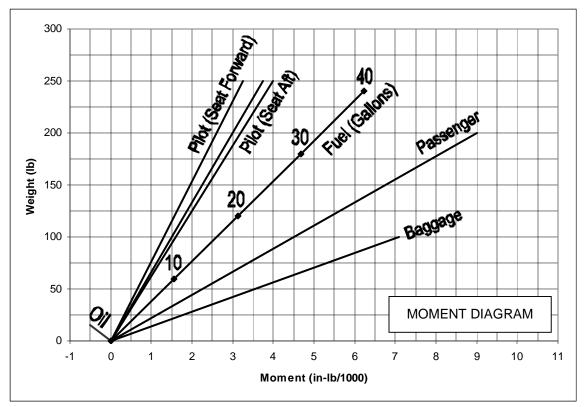
Add weights and moment of items in MOMENT DIAGRAM to airplane empty weight and moment (negative oil moment). Locate intersection of total weight and moment on AIRPLANE LOADING ENVELOPE. Any point falling within the envelope meets all balance requirements.
